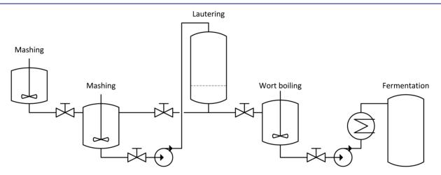
Figure 2. Principle of the pilot scale brewing system such as employed at Aalborg University, Esbjerg Campus.
