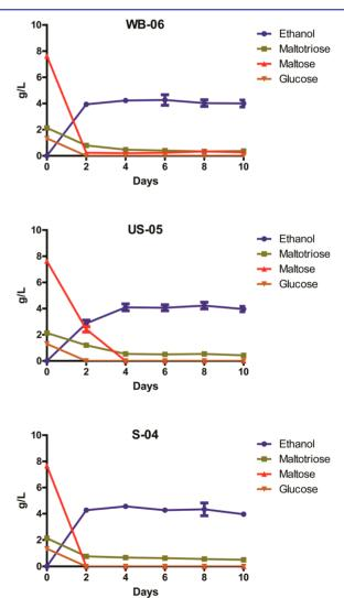
Figure 4. Changes in concentration of ethanol, maltotriose, maltose, and glucose (g/L) during 10 days fermentation of three different yeast strains (WB-06, US-05, and S-04) in malt extract medium. Three independent samples were analyzed at each time point for each strains and the data is shown as mean values with error bars representing standard deviation.
