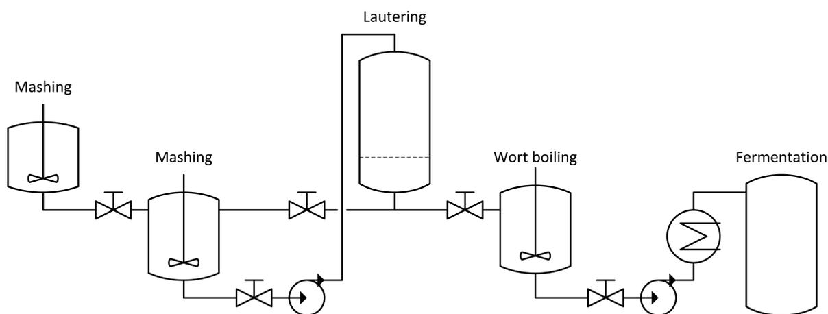
**Figure 2.** Principle of the pilot scale brewing system such as employed at Aalborg University, Esbjerg Campus.
