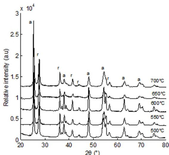
**Fig 1.** XRD patterns of titania-silica with varying calcination temperature. The wavelength of X-ray is 1.54056 Å. Legend: a = anatase and r = rutile
