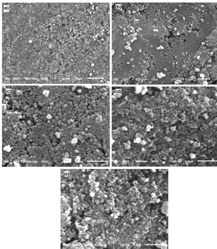
**Fig 3.** SEM images of samples with various calcined temperatures: (a) sample A at 500; (b) B at 550; (c) C at 600; (d) D at 650; and (e) E at 700 °C
