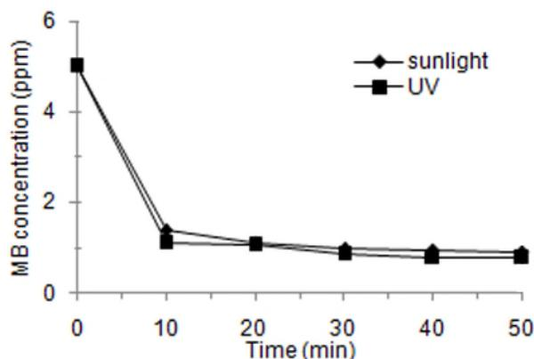
**Fig 4.** Decreasing MB concentration as a function of time under UV and Vis rays at 500 °C (sample A)
