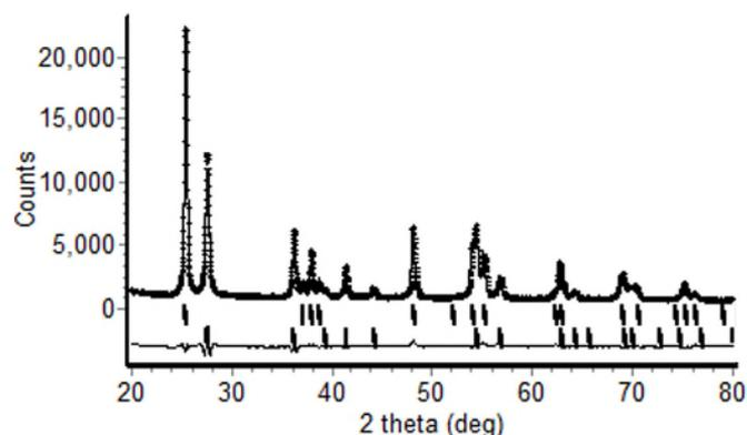
**Fig 2.** XRD profile for sample E at 700 °C. Measured and calculated patterns are indicated by crosses (black) and solid line, respectively. Intensity differences between the two patterns are shown along the bottom of the plot. Vertical bars represent the allowable peak position for each of the phases (from top to bottom: anatase and rutile)
