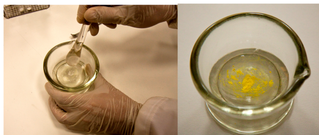
Figure 3. Change in color of the sample after using a mortar, from white to yellow.
