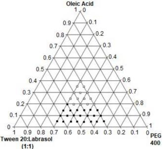
**Fig 2.** Pseudoternary phase diagram of SNEDDS consist of oleic acid, Tween 20:labrasol (1:1), and PEG 400
