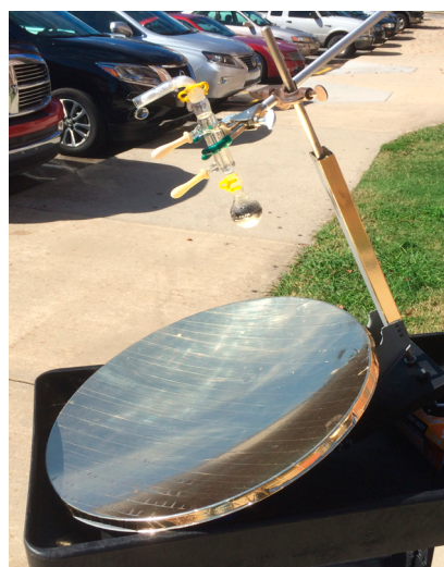
Figure 3. Solar experiment reaction setup using solar reflector.
