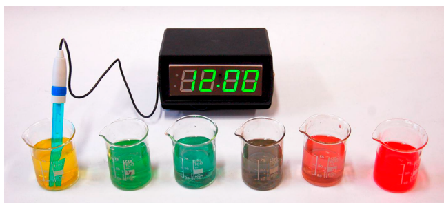
Figure 2. Setup of a demonstration pH meter with LED display of pH values.
