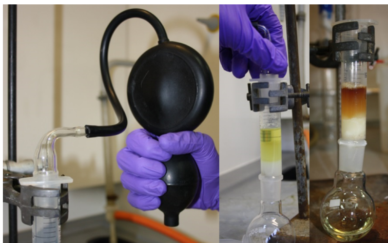
Figure 2. Photograph of silica gel column the students used to purify their product.
