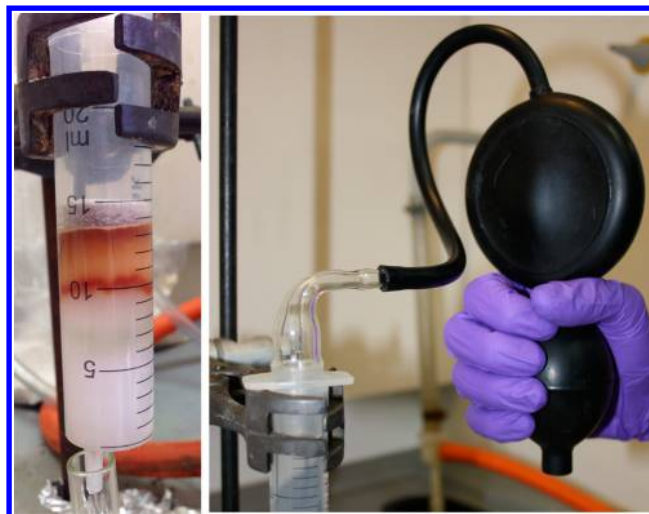
Figure 2. Photograph of silica gel column the students used to purify their product.
