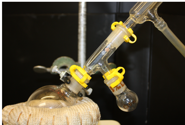
Figure 1. Dean–Stark trap, constructed from a stillhead and a 5 mL round-bottom flask, used at Abington campus.
