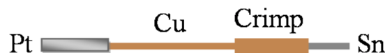
Figure 3. Mini-cell made from a Cu wire coated with Pt at one end and joined to a Sn wire at the other end by means of a copper crimp connector.
