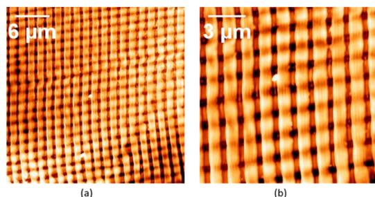
Figure 9. The 30  $\mu\text{m}$   $\times$  30  $\mu\text{m}$  (a) and 15  $\mu\text{m}$   $\times$  15  $\mu\text{m}$  (b) scans of PVP structures.
