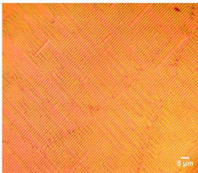
Figure 8. Optical images of PVP patterns magnified at 100 $\times$ .
