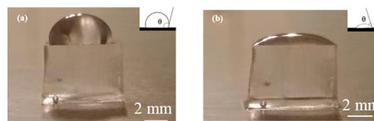
Figure 2. Drop of water on the surface of PDMS (a). Inset illustrates a contact angle ( $\theta$ ) greater than  $90^\circ$ . Drop of isopropyl alcohol on the surface of PDMS (b). Inset illustrates a contact angle ( $\theta$ ) less than  $90^\circ$ .
