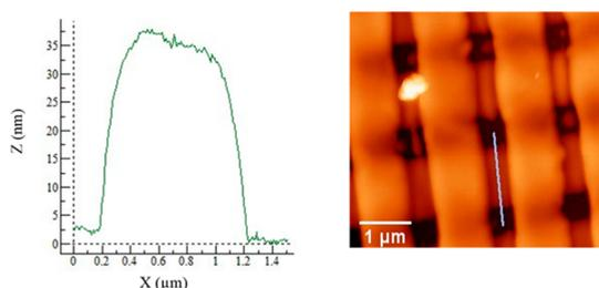
Figure 10. Cross-section plot (left) obtained from an AFM scan of PVP structures (right).
