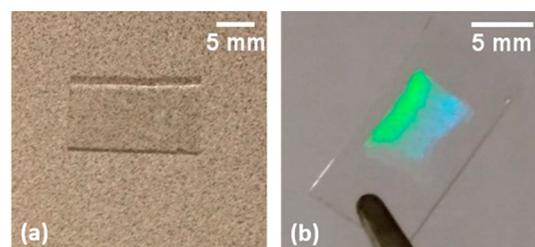
Figure 7. Transparency of deposited PVP film (a). Prismatic effect observed after stamping PVP pattern (b).
