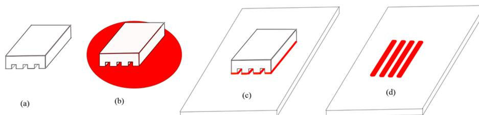
Figure 5. Diagram illustrating microcontact printing steps.
