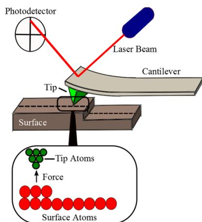
Figure 4. Diagram illustrating AFM operation.
