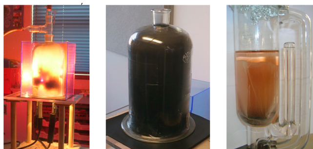
Figure 2. Left: The arcing process underway. Middle: Following arcing, the bell jar is coated with a crude, sooty product. Right: Close-up photograph of the Soxhlet extractor. The orange-red coloration is due to C_{70} , which was also formed by the arcing process, and which masks the magenta color of C_{60} in toluene.
