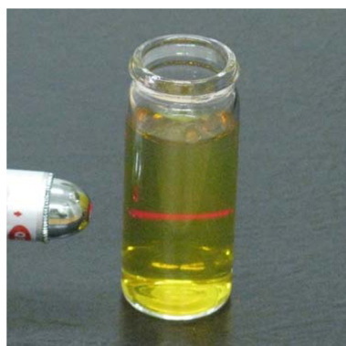
Figure 2. Visualization of a laser beam directed through the yellow sol of silver nanoparticles.
