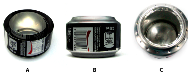
Figure 2. The support is placed in the middle of the base (A); the cover over the base and support forms the burner (B); and top view of burner with the pinholes along its top frame (C).
