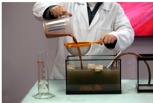
Figure 2. Beaker containing gravel and part of the wastewater (here, clay) is poured into the kitchen sieve in order to retain the gravel.
