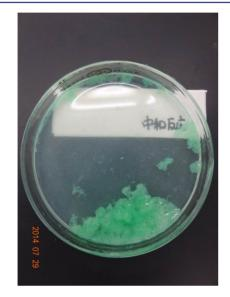
Figure 3. Slime (No. 5, Table 1) dissociated with sat. NaHCO<sub>3</sub> to form small lumps with the release of  $CO_2$ .
