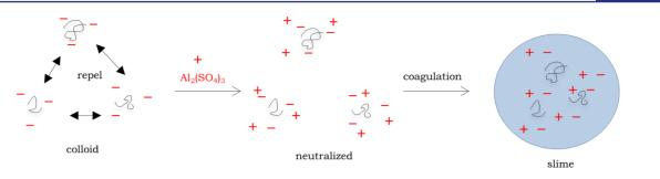
Figure 2. Coagulation mechanism.
