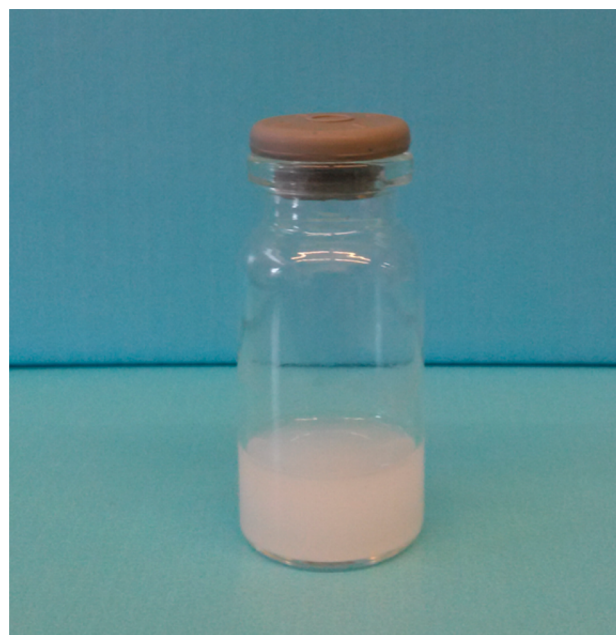
Figure 1. Colloidal suspension of PLGA NPs prepared by the single emulsion–solvent evaporation method.
