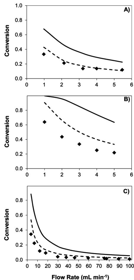
Figure 3. Experimental conversion ( $\blacklozenge$ ) obtained for (A) CSTR, (B) PFR, and (C) FBR at different flow rates and respective modeling using the enzyme intrinsic kinetic constants (—) and the apparent kinetic constants (---). Initial concentration of sucrose was 10 g $\cdot$ L<sup>-1</sup>. Concentration of biocatalyst was 500 mg cells $\cdot$ g Alginate<sup>-1</sup>. Working volume  $\approx$ 10 mL for all reactors. Studies were performed at 45 °C and pH 4.5.
