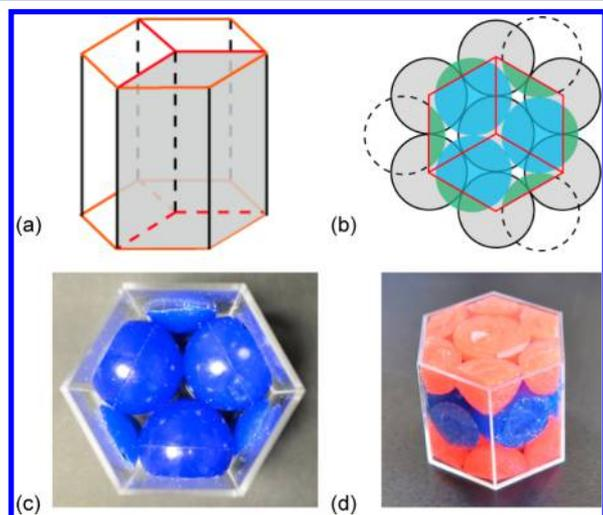
**Figure 5.** (a) The rhombus unit cell and hexagonal unit, (b) projection of the hcp structure viewed along the hexagonal axis, (c) packing mode of the second layer in the hexagonal unit, and (d) the hcp structure in a hexagonal unit.
