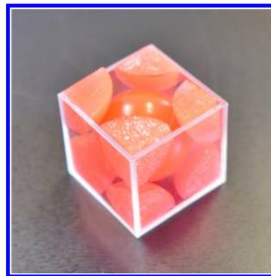
**Figure 6.** Unit cell structure of the bcc structure.
