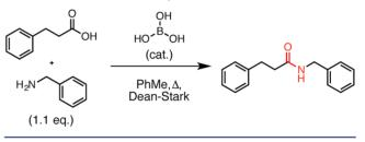
Boric acid catalyzes amide-bond formation between carboxylic acids and amines at elevated temperatures.<sup>25</sup> The hydrocinnamic acid, benzylamine, and amide product all have reaction stoichiometry coefficients of 1, though in practice the amine is used in slight excess (see the Supporting Information). The prelab discussion addresses the catalytic mechanism, and describes the proper use of a Dean–Stark trap since water must be removed from the mixture over the course of the reaction.
