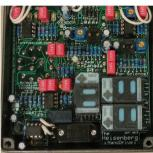
The Heisenberg Molecular Overdrive creates distortion on electric guitar sounds. It gets its warm sound from molecular junctions, built into SIM cards in the effects pedal's circuit board. Credit: Adam Bergren.
