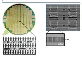
Researchers have harnessed carbon nanotubes to build computer circuits. This 100 mm wafer is patterned with circuit elements made of individual carbon nanotubes. Layering nanotubes over silicon elements could improve chip performance. Credit: Max M. Shulaker.
