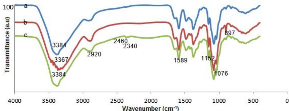
**Fig 3.** FT-IR spectra of chitosan (a), chitosan-silica membrane (b), and chitosan-silica-dithizone membrane (c)
