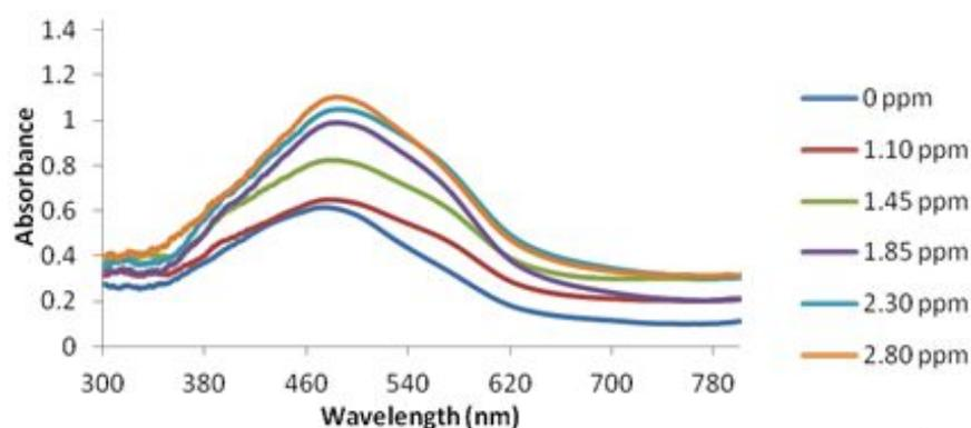
Fig 6. Absorbance spectra of proposed optode at various concentrations of  $Pb^{2+}$  ion solution
