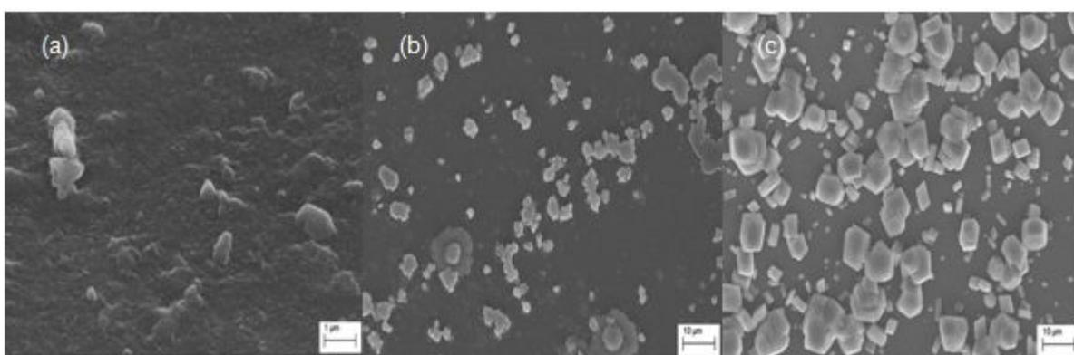
**Fig 4.** Electron microscopy image of chitosan membrane (a), chitosan-silica membrane (b), and chitosan-silica-dithizone membrane (c)
