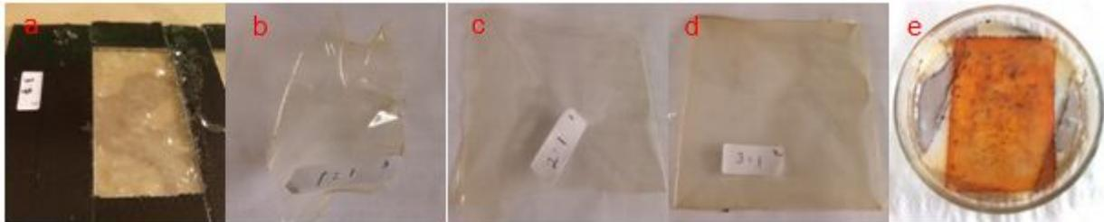
**Fig 1.** Membranes with various volume ratio of chitosan-silica of 3:7 (a), 1:1 (b), 2:1 (c), 3:1 (d), and chitosan-silica membrane ratio of 2:1 after immobilization of dithizone (e)
