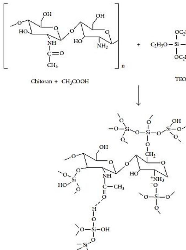
**Fig 2.** Schematic structure model of chitosan-silica membrane
