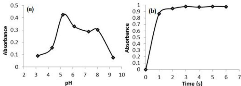
Fig 7. Effect of pH (a) and contact time of sensor (b) against the absorbance
