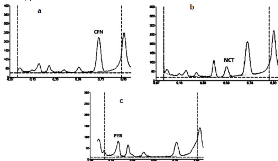
Fig 2. Chromatograms of the energy drinks sample (a) UV detection at 274 nm, (b) UV detection at 263 nm, and (c) UV detection at 293 nm. Chromatographic conditions: mobile phase, methanol-ethyl acetate-ammonia 25% 13:77:10 (v/v/v); CFN: caffeine; NCT: nicotinamide; PYR: pyridoxine
