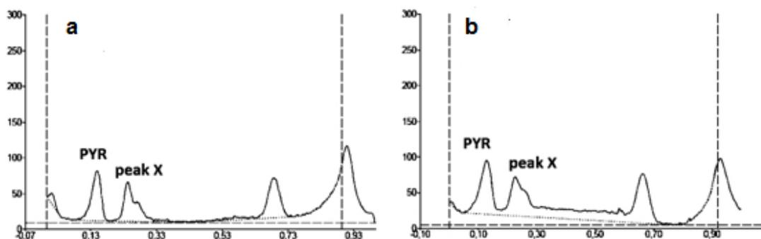
**Fig 3.** The effect of shortening the elution distance on the pyridoxine selectivity (a) Elution distance 75 mm (Resolution 1.29), (b) Elution distance 50 mm (Resolution 0.95). Chromatographic conditions: mobile phase, methanol-ethyl acetate-ammonia 25% 13:77:10 (v/v/v); PYR: pyridoxine
