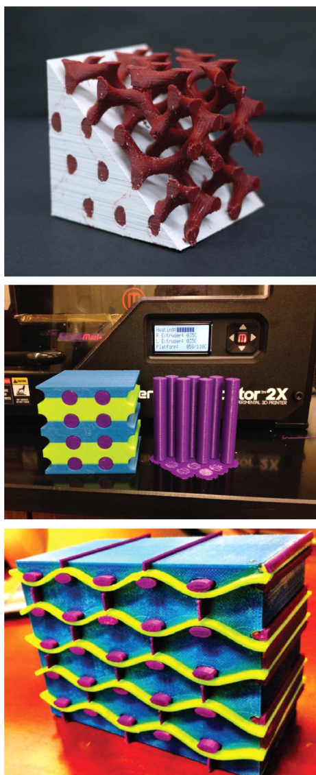
Figure 3. Close-up photograph of the 3D printed AB diblock gyroid (G) morphology (top). 3D printed ABC triblock copolymer self-assembled morphology and B cylinders at A/C lamellar interface (middle), and the ABC triblock copolymer knitting pattern (bottom). The structures were 3D printed in ABS plastic with approximate dimensions of 8 cm in all directions.
