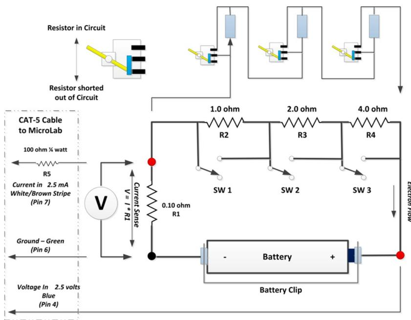
**Figure 2.** Circuit diagram of the resistive load module. The module included a set of four resistors, three of which could be switched in or out to provide variable resistance. The current through the circuit was determined by measuring the voltage drop across resistor R1. See Supporting Information for more details.
