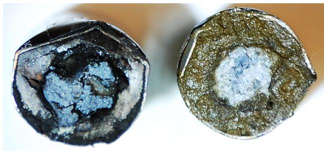
**Figure 1.** Cross-sectional view of a fresh (left) and spent (right) Duracell alkaline battery. The inner (anode) portion contains Zn, ZnO, or both in KOH electrolyte in a gel; the outer (cathode) portion contains MnO<sub>2</sub>, MnOOH, or both in conductive carbon. The anode and cathode are separated by a porous membrane.
