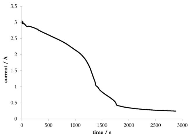
**Figure 3.** Current vs time observed for a Duracell AA alkaline battery that was almost completely drained using the MicroLab RLM.
