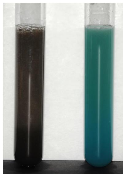
**Figure 8.** Material from the cathode of a fresh (left) and spent (right) Duracell alkaline battery added to a mixture of methylene blue and H<sub>2</sub>O<sub>2</sub>. Strong effervescence and rapid discoloration of methylene blue catalyzed by fresh cathode indicates the presence of MnO<sub>2</sub> rather than reduced Mn species.
