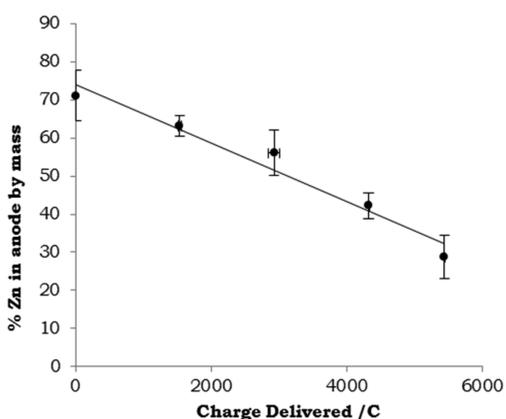
**Figure 6.** Percent Zn remaining in the anode for Duracell AA alkaline batteries discharged to varying extents.  $R^2 = 0.96$  for the linear fit (data pooled from several student trials).
