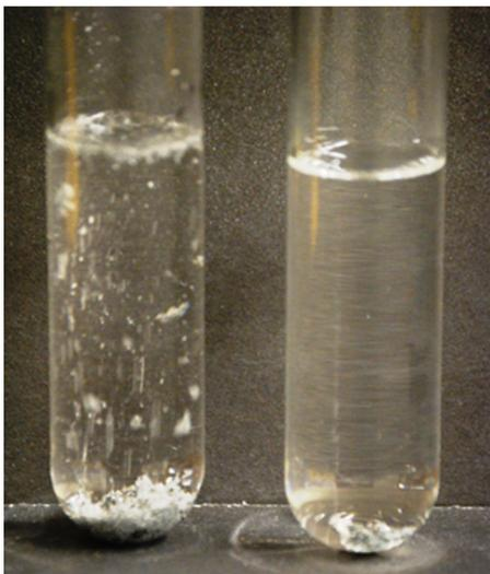
**Figure 7.** HCl (3 M) added to anodic material from a (left) fresh and (right) spent Duracell alkaline battery. The substantially greater bubbling observed in the former is indicative of a much higher Zn content in the fresh battery.
