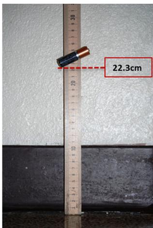
**Figure 4.** Measurement of battery bounce height.
