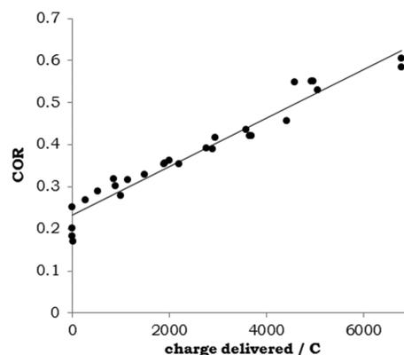
**Figure 5.** COR for Duracell AA alkaline batteries discharged to varying extents.  $R^2 = 0.95$  for the linear fit (data pooled from several student trials).
