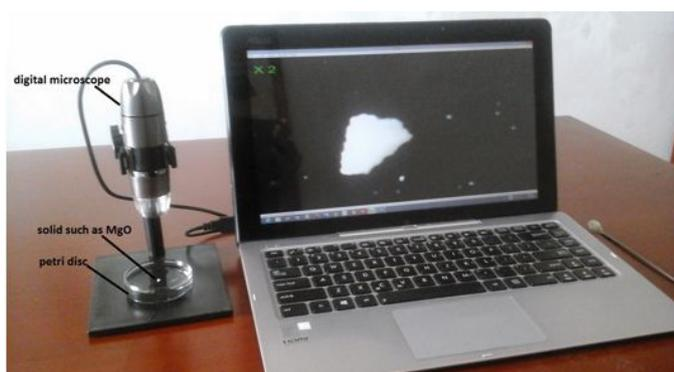
Fig 2. Arrangement of the solid-liquid chemical reaction observation kits
