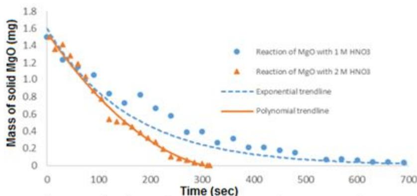
**Fig 6.** Plot of MgO mass against reaction time observed using a microscope and processed using the application with different concentration of  $\text{HNO}_3$
