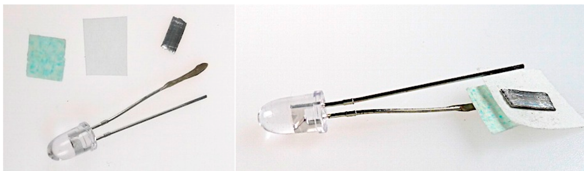
Figure 1. Three galvanic cell components and a LED shown separate (to the left) and oriented for assembly (to the right). The three cell components are (from the left) a piece of paper with copper sulfate, a piece of paper with sodium sulfate, and a piece of magnesium ribbon. Notice that the positive terminal of the LED is coated with a conductive glue.
