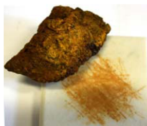
Figure 2. Streak plate revealing the characteristic yellow-brown streak of limonite (the compound color in powdered form).
