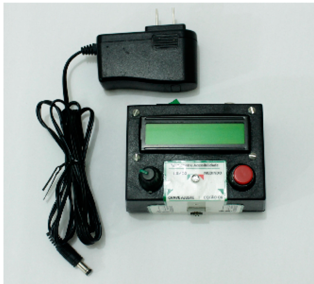
Figure 3. Accessibility thermometer controller.
