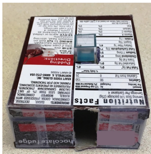
Figure 3. A cardboard box cut to fit sample. Note the rectangle cut in the front of the sample box to allow the cell phone camera to detect light passing through the sample. The entire back panel of the box has been removed to allow light from a source to pass through the sample.
