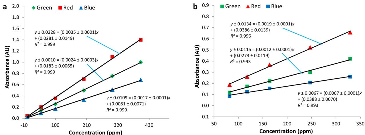
**Figure 6.** Calibration curves for phosphate using (a) the Murphy–Riley method and (b) the modified Murphy–Riley method, and the custom-built colorimeter.
