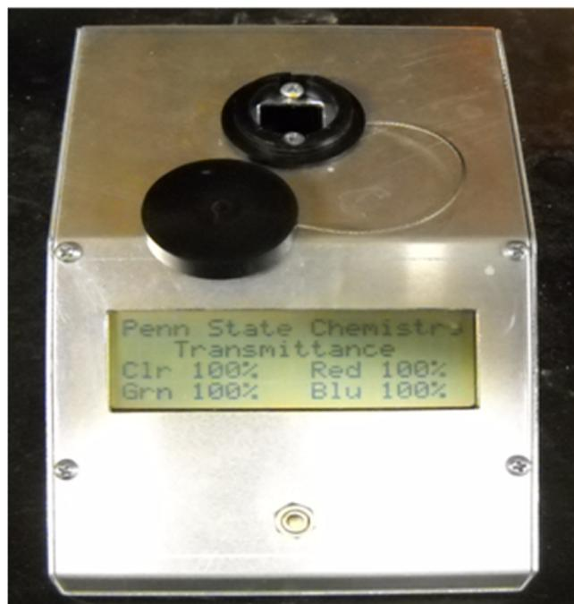
Figure 1. Custom-built colorimeter.
