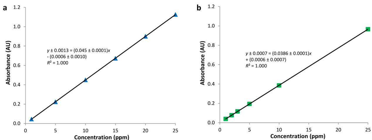
Figure 3. Calibration curves at  $\lambda_{\max}$  for (a) tartrazine (427 nm) and (b) amaranth (521 nm) using a Cary-4000 commercial spectrometer.
