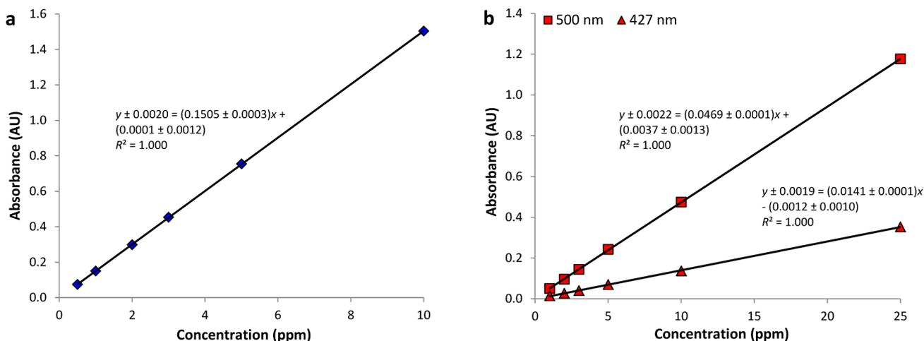
Figure 5. Calibration curves at  $\lambda_{\max}$  for (a) Blue 1 (629 nm) and (b) Red 40 (427 and 500 nm) using a Cary-4000 spectrometer.
