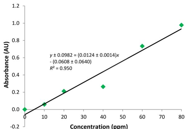
**Figure 7.** Calibration curves for Fe–salicylate using the custom-built colorimeter at 524 nm. The anomalous data point at 40 ppm is real and a consequence of error introduced by the students during standard preparation; deleting this point gives an  $R^2$  value of 0.999.
