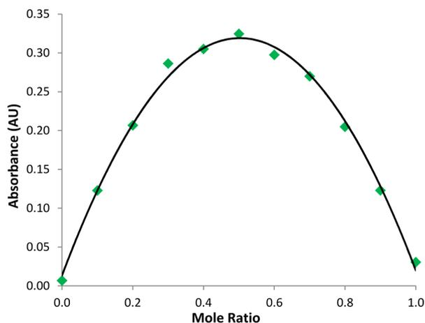
**Figure 8.** Method of continuous variation plot for the iron–salicylate complex using the custom-built colorimeter at 524 nm.
