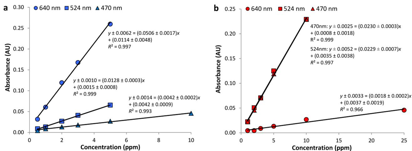
**Figure 4.** Calibration curves for (a) Blue 1 and (b) Red 40 using the custom-built colorimeter.
