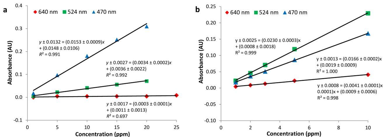
Figure 2. Calibration curves for (a) tartrazine (Yellow 5) and (b) amaranth (Red 2) using the custom-built colorimeter.
