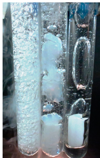
Figure 3. Bubble sizes observed when dry ice is added to liquids. Ethanol (left tube), water (center tube), and room temperature glycerin (right tube). Small bubbles indicative of nucleate state sublimation also form in acetone, hexane, methanol, and isopropyl alcohol (data not shown).
