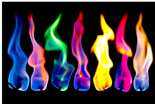
Figure 1. Flames generated by igniting sponges soaked in mixtures of methyl alcohol and metal salts as described in ref 5. Sponge soaked in methyl alcohol and (L to R) no salt, calcium nitrate, copper(II) nitrate, strontium nitrate, sodium nitrate, lithium nitrate, and potassium nitrate. Image created by Christopher Burleson and reprinted with permission.
