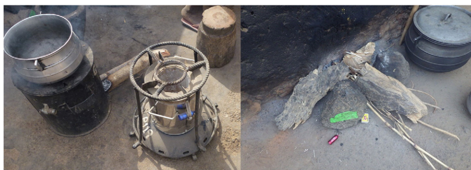
Fig. 2. Digit-TL SUM placements on the Gyapa, Philips, and 3-stone fires, from left to right. The Philips stove is shown with the specially designed rebar pot stand. The 3-stone fire at right is shown with wood and millet stalks for fuel.
