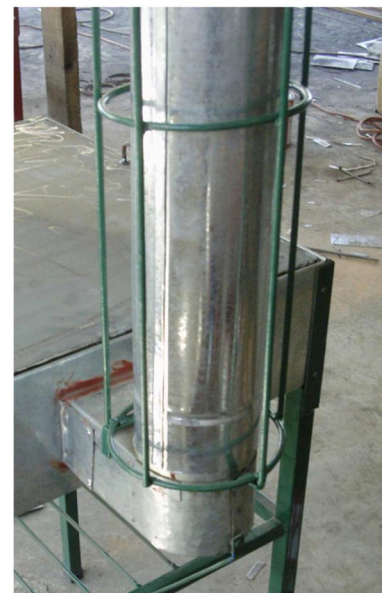
Fig. 6. Shielding surrounding the chimney to reduce the chance of contact with skin.
