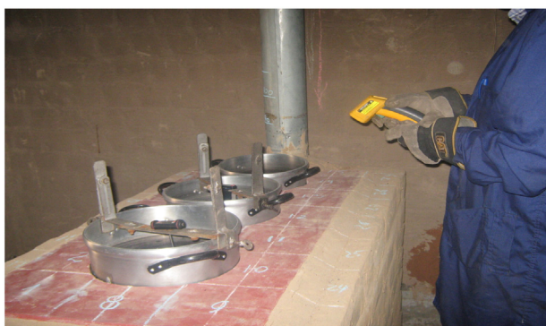
Fig. 5. Chalk grid marked along the exterior of the cookstove for the surface temperature test. Photo courtesy of Laboratory of Evaluation of Stoves SENCICO.
