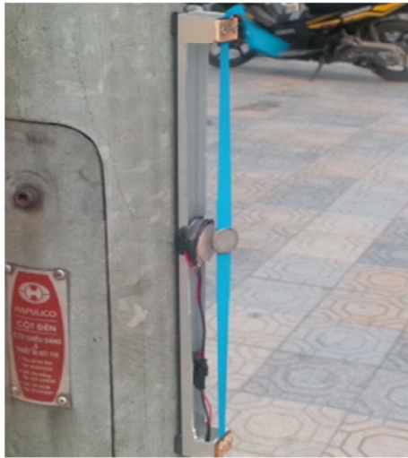
Fig. 20. Testing the single membrane generators in outdoor condition.
