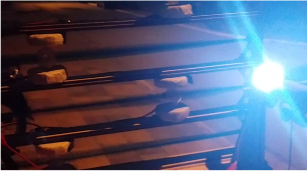
Fig. 24. Testing of the windpanel powering a LED light in real wind condition.
