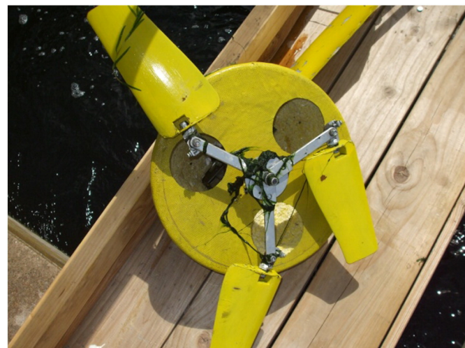
Fig. 11. Blades virtually weed-free but some weed still wrapped around the shaft.
