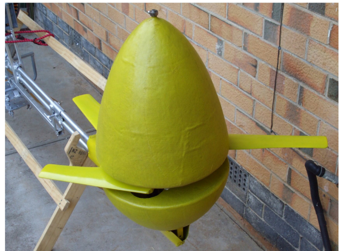
Fig. 10. Modified turbine with larger nose cone (below) and tail cone (above), showing a blade swung back in nearly tangential orientation to facilitate self-cleaning.
