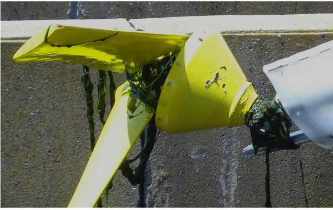
Fig. 7. Weed/algae tangled in turbine hub and gearbox.
