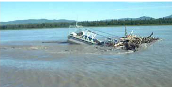
Fig. 2. Driftwood on hydrokinetic turbine pontoon and anchor cable in Alaska (Tyler, 2011).
