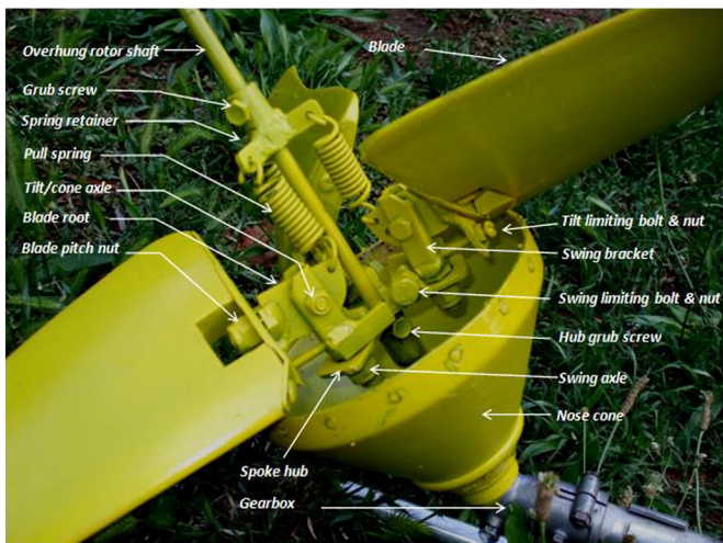
Fig. 5. Hub as originally constructed, complete with coning and swinging mechanisms, blade pitch adjustment and nose cone (nacelle).
