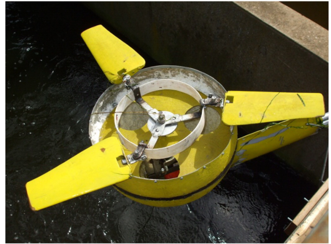
Fig. 12. Final design with ring behind the nose cone to prevent weed winding around the shaft made the turbine remained virtually weed-free.
