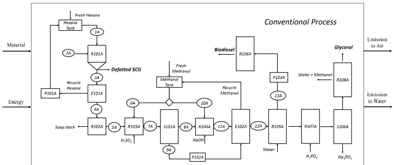
Fig. 2. System boundary of conventional SCG biodiesel production at a central facility.
