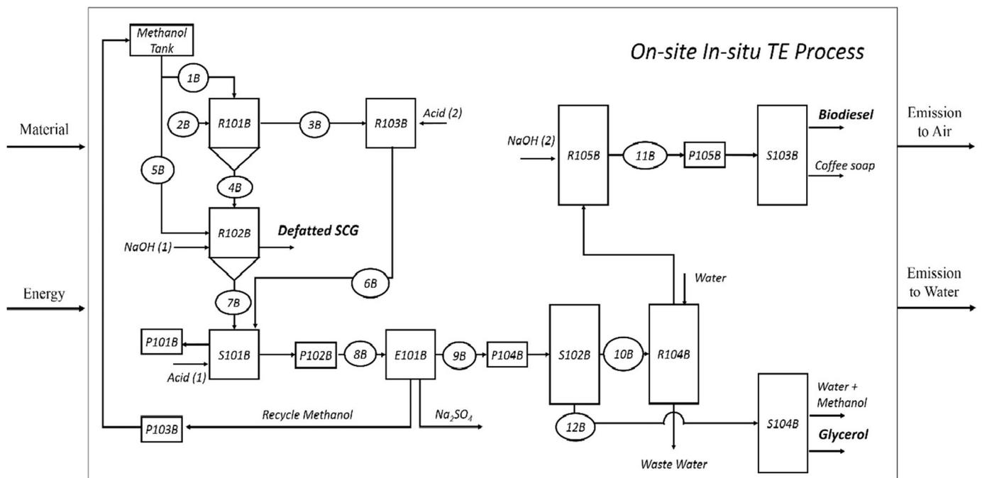
**Fig. 3.** System boundary of the on-site SCG biodiesel production process.
