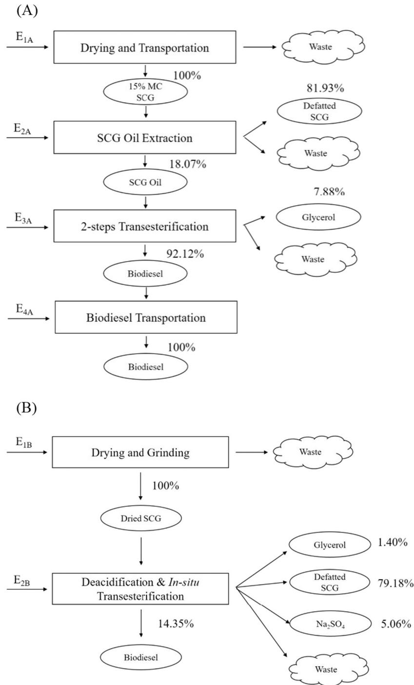
Fig. 4. Mass-based allocation of biodiesel and its by-products from the conventional (A) and on-site *in-situ* TE processes (B).
