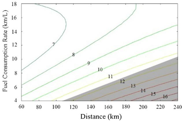
Fig. 6. Energy usage (MJ/kg biodiesel) of conventional processing at various transportation distances and vehicle fuel consumption rates; the shade area indicates the conditions that have energy usage that exceeds that of an on-site *in-situ* TE processing (11.38 MJ/kg biodiesel).
