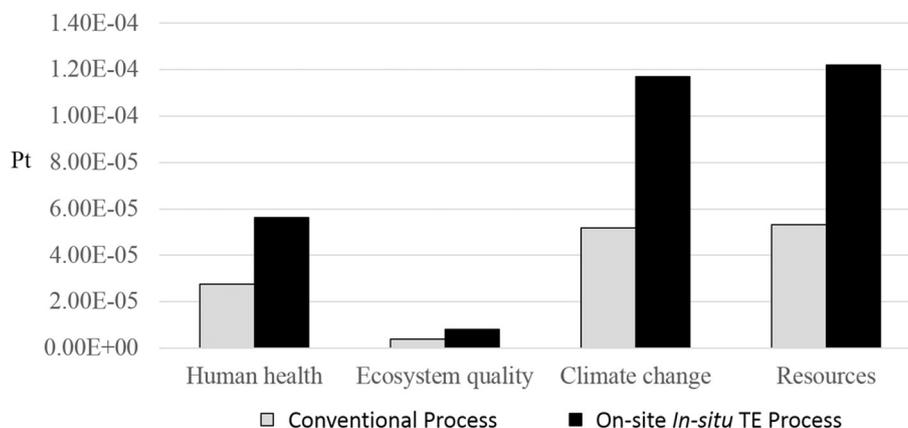
**Fig. 10.** Comparison of the single-score environmental impacts of producing SCG biodiesel *via* the conventional and on-site *in-situ* TE processes, according to IMPACT 2002+. Functional unit: 1 kg biodiesel. Units correspond to points (Pt).
