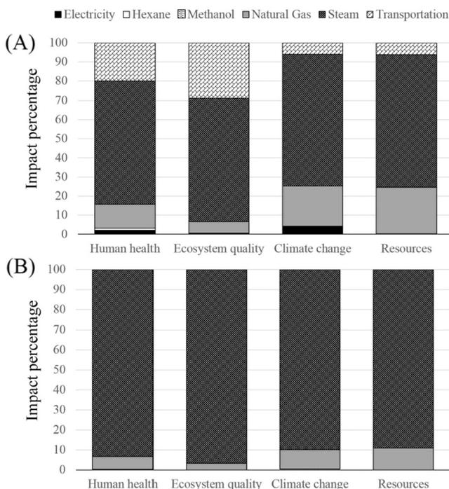
Fig. 9. Relative endpoint environmental impacts of conventional (A) and on-site *in-situ* TE (B) processes based on energy form and solvent leaking from the system, according to IMPACT 2002+.
