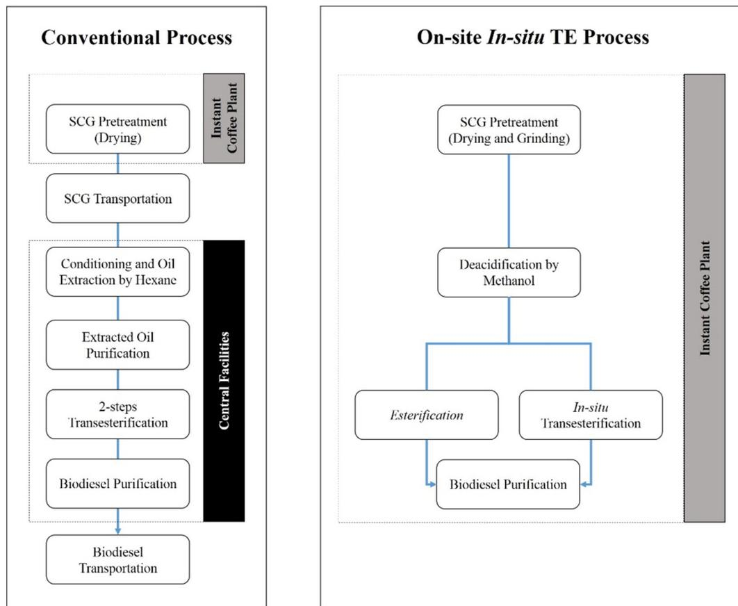
Fig. 1. A comparison of conventional and on-site *in-situ* TE SCG biodiesel process steps.
