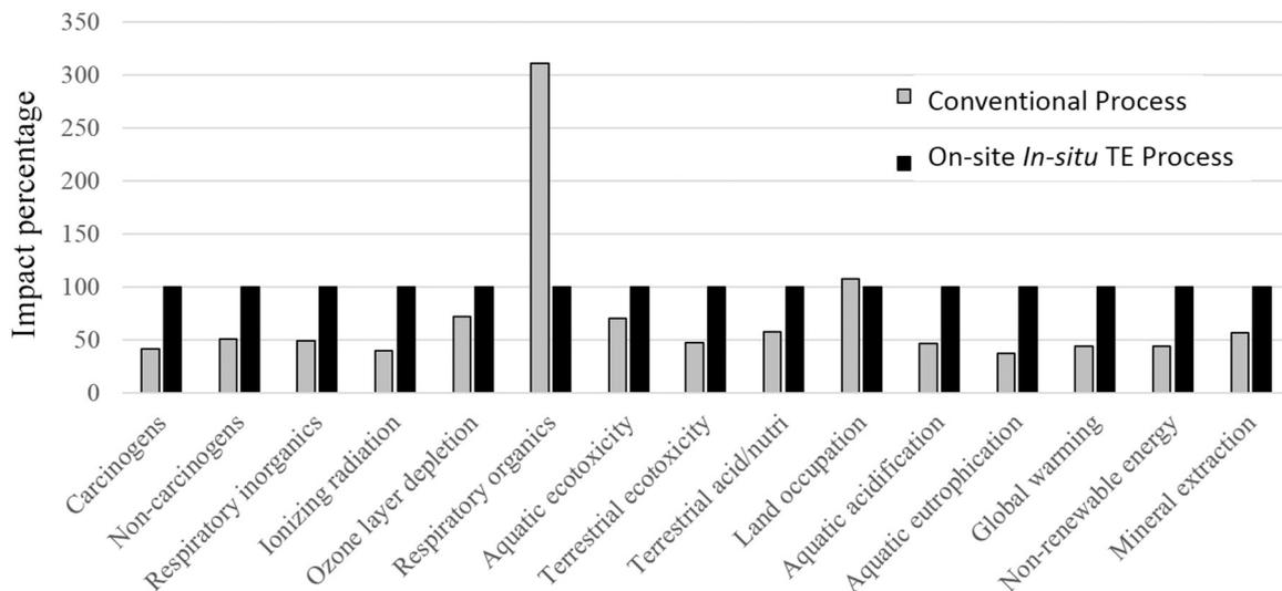
Fig. 7. Relative midpoint environmental impacts of SCG biodiesel produced by conventional and on-site *in-situ* TE processes according to IMPACT 2002+.
