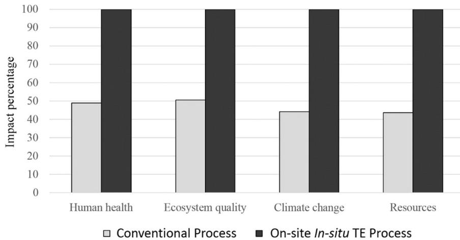
Fig. 8. Relative endpoint environmental impacts of SCG biodiesel produced by conventional and on-site *in-situ* TE processes according to IMPACT 2002+.
