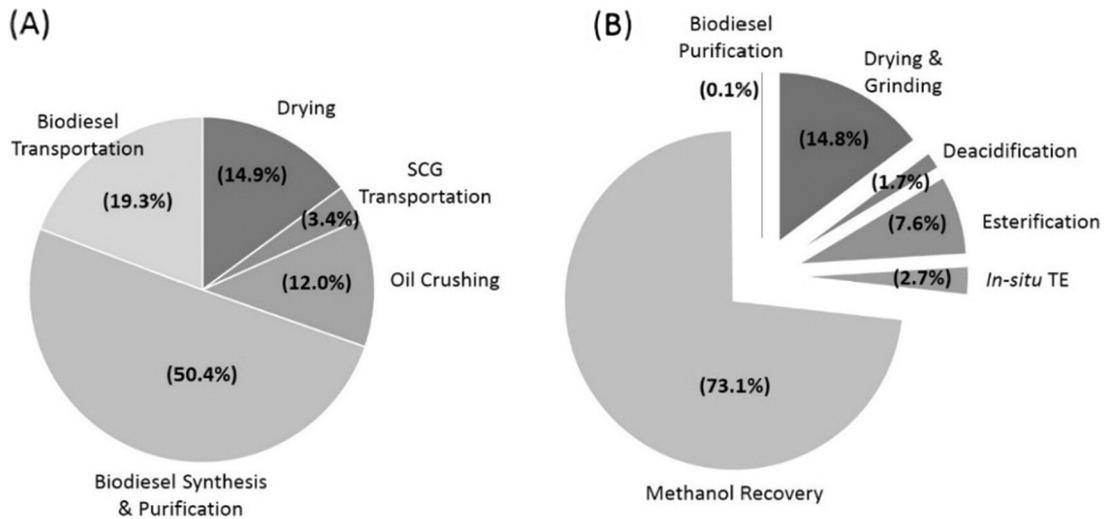
Fig. 5. Percentage of energy usage of each sub-process in the conventional (A) and on-site *in-situ* TE processes (B). The energy usages of the conventional and on-site *in-situ* TE processes were 6.49 and 11.38 MJ/kg biodiesel, respectively.
