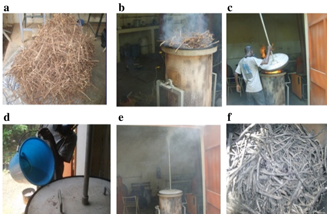
Fig. 3. Description of the stages of carbonization: (a) chopped cotton stalks, (b) end of filling of the reactor and the beginning of the combustion time, (c) reactor closing and end of the combustion time, (d) sealing by introduction of water into the throat, (e) smothering of the combustion and cooling the charcoal, (f) cotton stalks charcoal.
