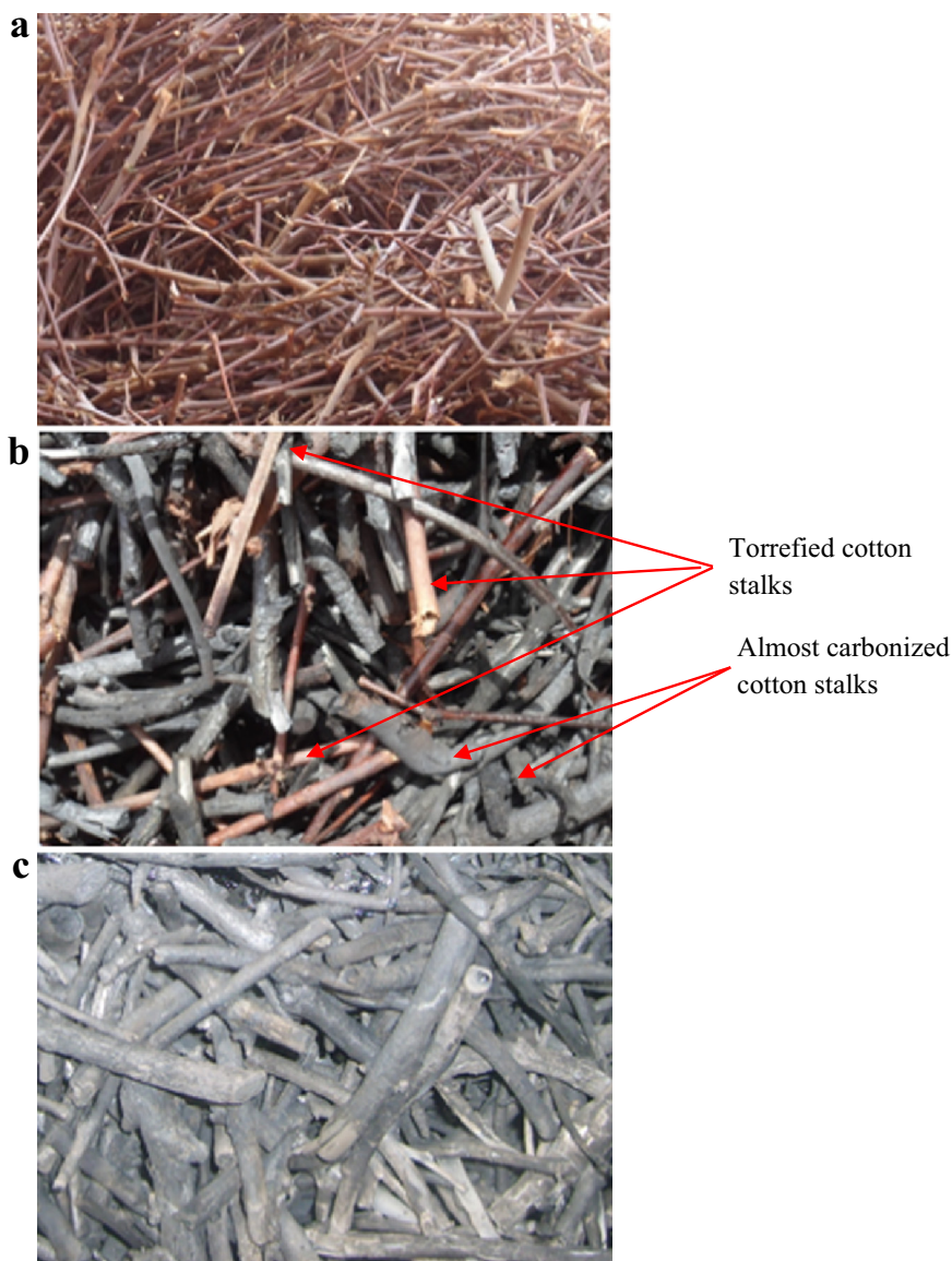
Fig. 6. Raw cotton stalk and residues from carbonization and torrefaction of cotton stalks by partial combustion. (a) Raw cotton stalk; (b) Torrefied cotton stalks; (c) Carbonized cotton stalks.
