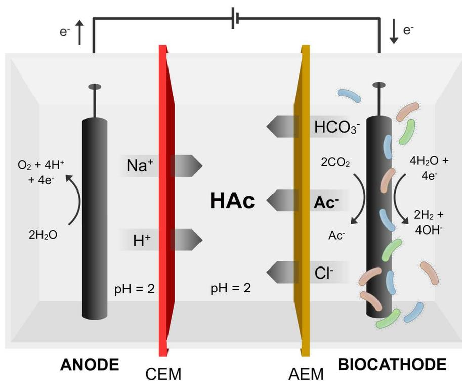
Reactor concept for simultaneous biological production and extraction of acetate from CO<sub>2</sub> and electrical current. An anion exchange membrane (AEM) separates the cathode and extraction compartment. A cation exchange membrane (CEM) separates the anode and extraction compartment. The middle compartment serves as extraction compartment for recovery of acetate as acetic acid.
