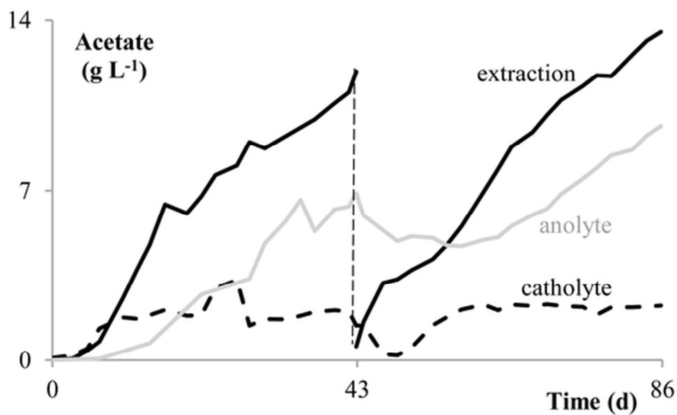
The acetate concentration ( $\text{g L}^{-1}$ ) in the extraction compartment steadily increased for a stable concentration in the cathode compartment. Concentrations in the catholyte (black dotted line), extraction compartment (full black line) and anolyte (grey line) are represented for a 86 day experiment. The vertical dotted line shows the start of the second cycle for the extraction compartment.
