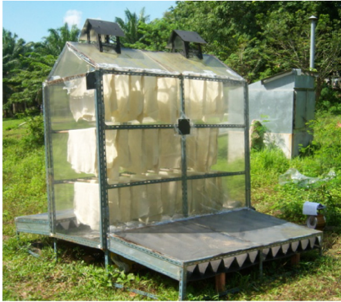
(a) Mixed-mode solar dryer for natural rubber drying
