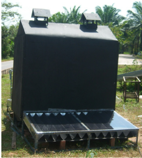
(b) Indirect solar dryer for natural rubber drying
