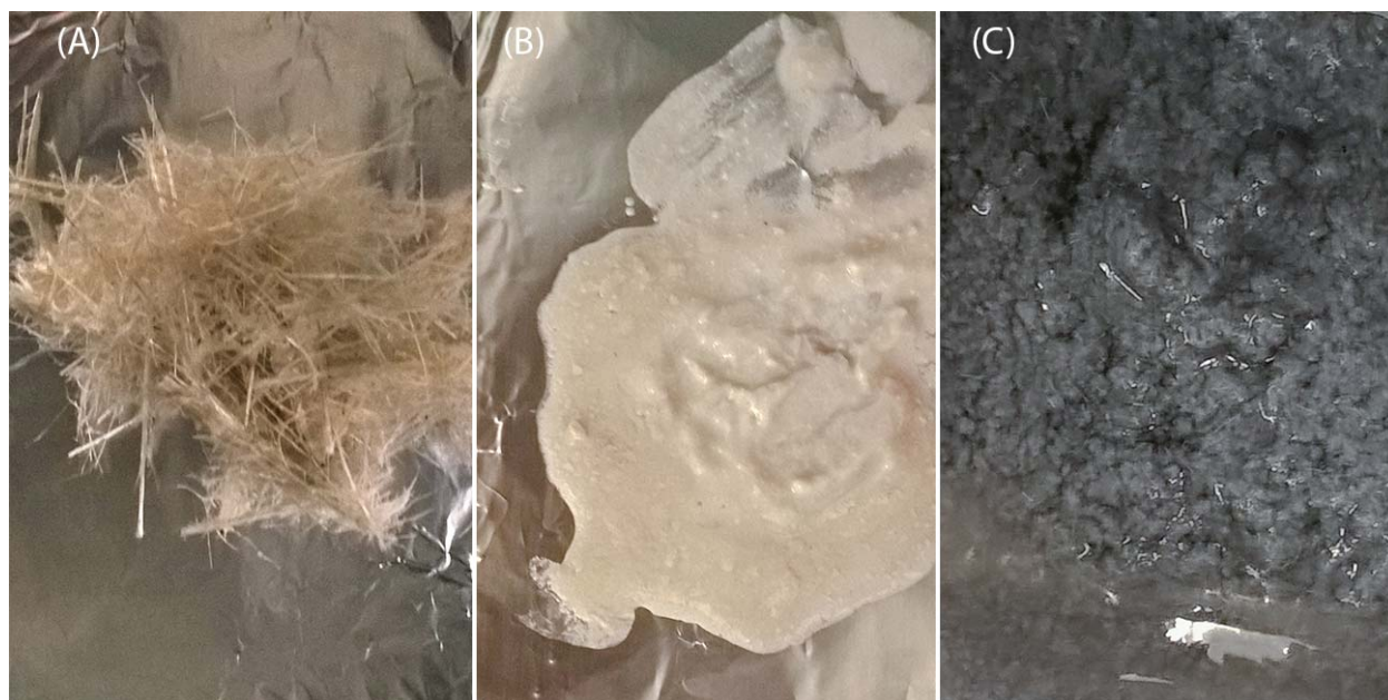
Figure 1. Grinding of chrysotile fiber bundles (A) with or without water affected the color of fibers produced. Drying grinding produced typical white fibers (B) whereas wet grinding produced gray fibers (C). The dry-ground fibers were soaked in water before the picture was taken.
