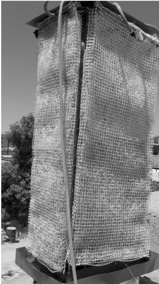
Fig. 5. A view of the constructed wind tower head with wetted surfaces.
