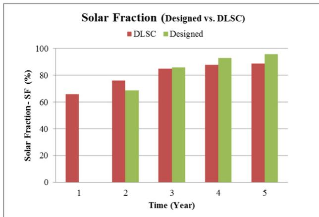
Fig. 11. Solar fraction comparison, DLSC vs. proposed system.
