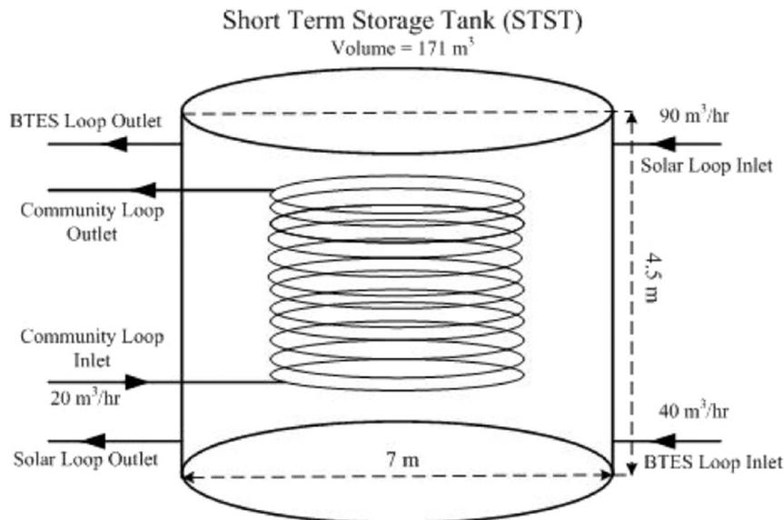
Fig. 6. Simplified schematic of short term storage tank.
