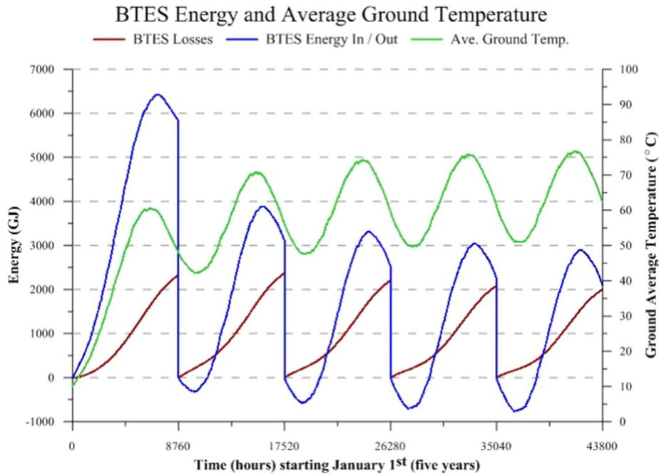
Fig. 7. BTES system accumulated energy and average temperature.
