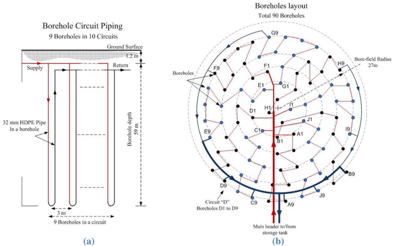
Fig. 5. (a) Borehole circuit piping schematic, (b) borehole field layout.
