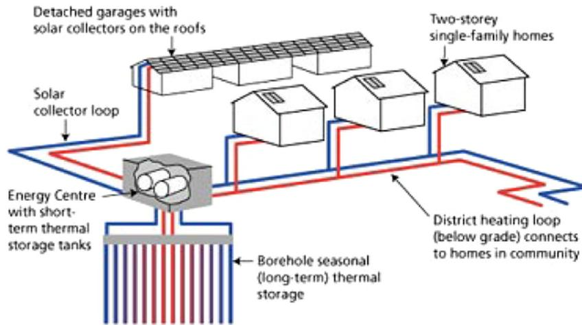
Fig. 1. Drake Landing Solar Community (DLSC) simplified system schematic (Nordell, 2000).
