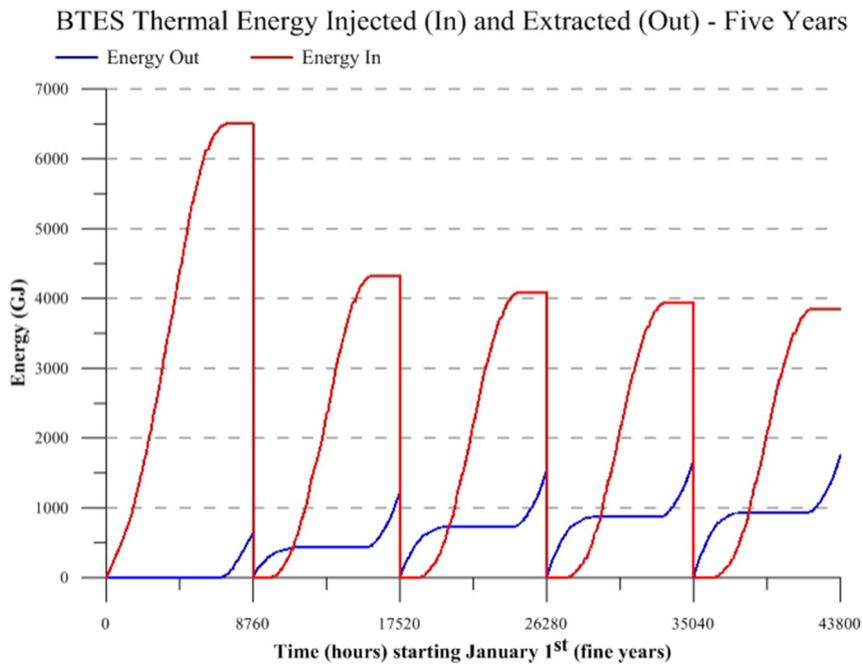
Fig. 8. Annual accumulated thermal energy injected into and extracted from the BTES.
