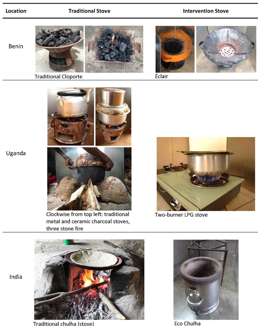
Fig. 1. Traditional and intervention stoves in Benin, Uganda, and Gujarat, India.
