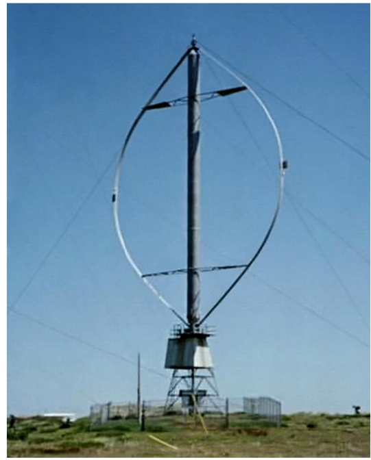
Fig. 12. Original troposkein curved blade Darrieus wind turbine: very little parasitic drag.
