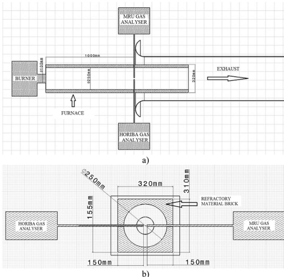
Fig. 3. The gas analysers positioning.
