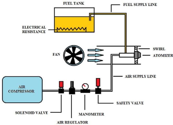
Fig. 2. Burner functioning scheme.
