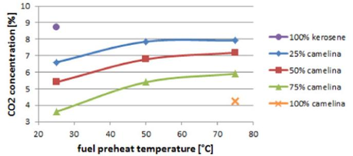
Fig. 7. CO<sub>2</sub> concentration in the exhaust gas function of fuel preheat temperature and of the fuel composition.
