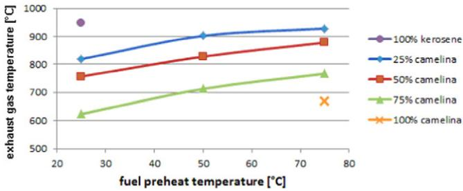
Fig. 5. Exhaust gas temperature function of fuel preheat temperature and of the fuel composition.
