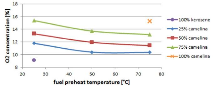
Fig. 8. O<sub>2</sub> concentration in the exhaust gas function of fuel preheat temperature and of the fuel composition.
