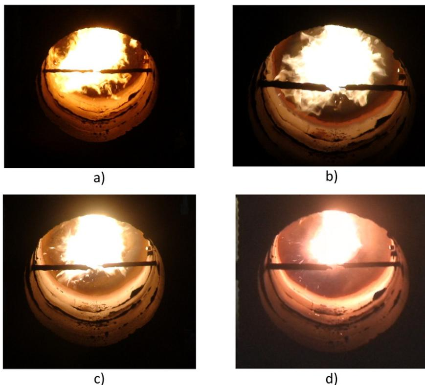
**Fig. 4.** The interior of the furnace while the burner was fuelled with: (a) 100% kerosene at 25 °C; (b) 25% camelina/75% kerosene at 25 °C; (c) 50% camelina/50% kerosene at 25 °C; (d) 75% camelina/25% kerosene at 25 °C.
