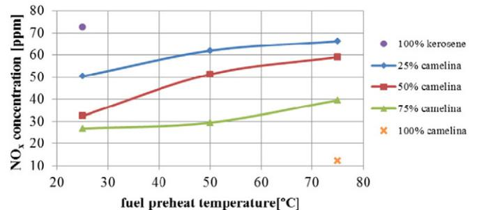
Fig. 9. NO<sub>x</sub> concentration in the exhaust gas function of fuel preheat temperature and of the fuel composition.
