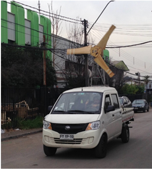
Fig. 3. 1 KW Wind turbine @ 6 m/s wind speed.
