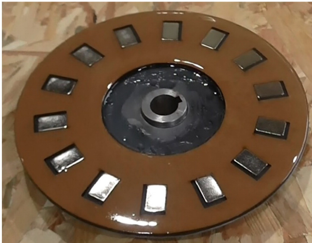
Fig. 7. Rotor dish with 14 permanent magnets.
