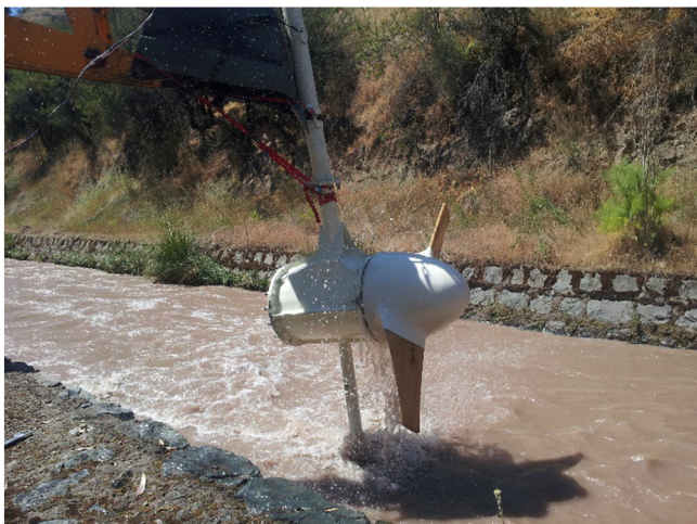
Fig. 4. Tidal turbine tested in an irrigation channel.
