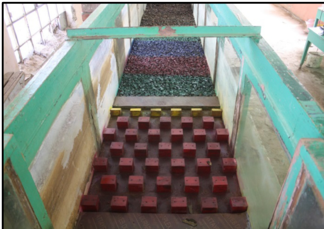
Fig. 6. The 2D physical model of spillway of a new Assiut barrage showing the installed baffle blocks.
